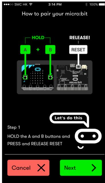
1. HOLD A & B buttons, at the same time PRESS and RELEASE RESET
