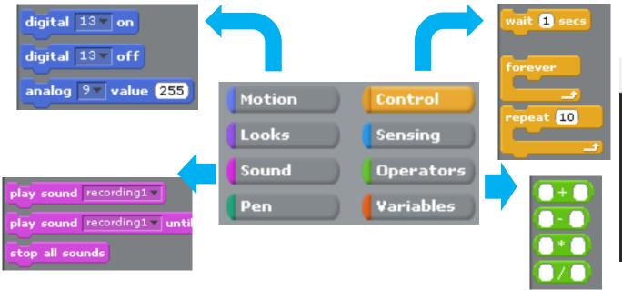
To upload codes to Arduino, one can use ArduBlock
