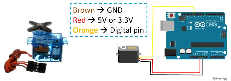
To control servomotor, one can download and install the library "Servo.h"
