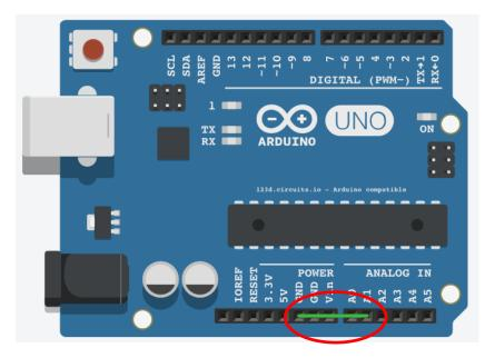
Analog input is a high impedance input, almost draw no current
